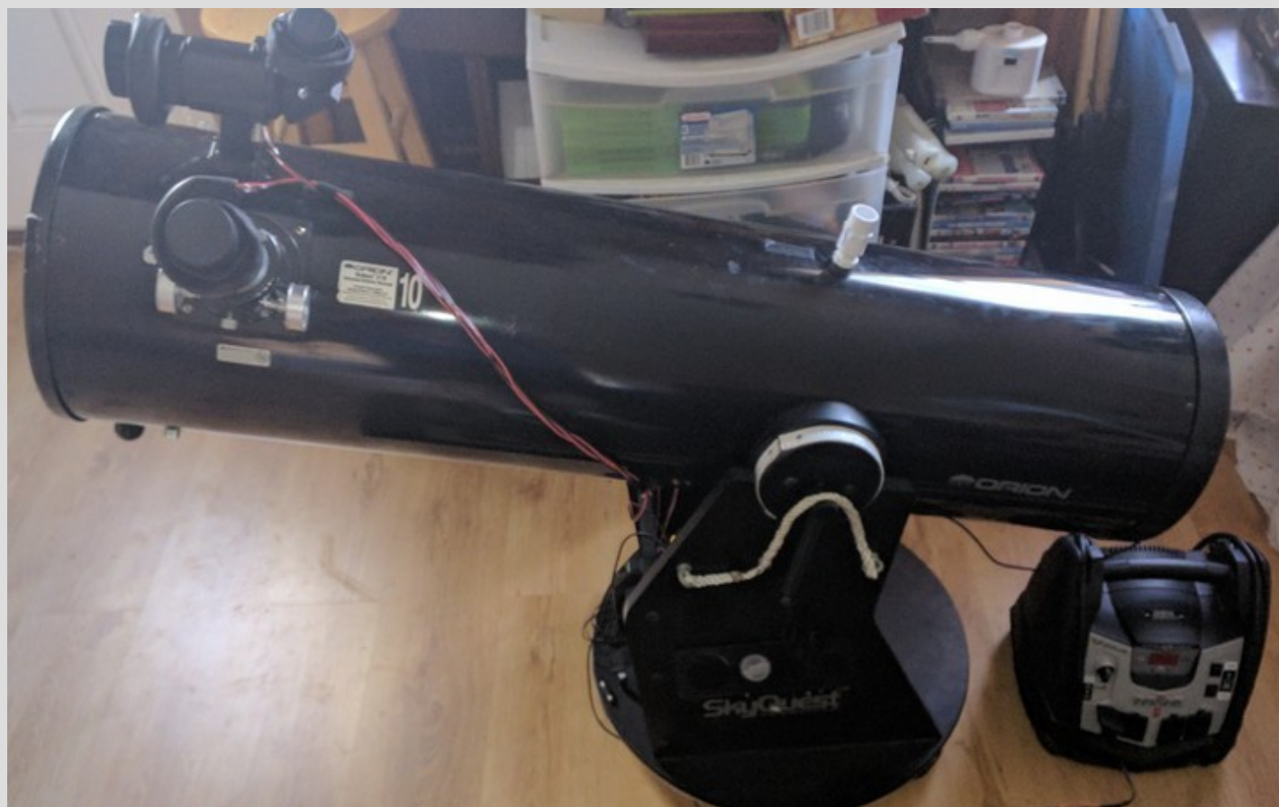
Illustration 72: Dew heaters installed
