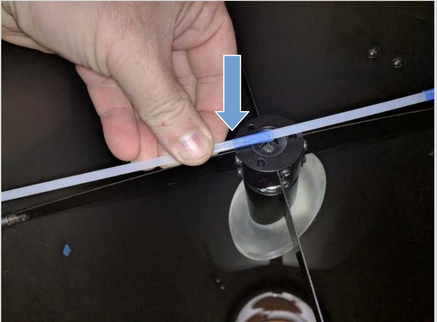
Illustration 25: Center secondary with plastic zip tie
